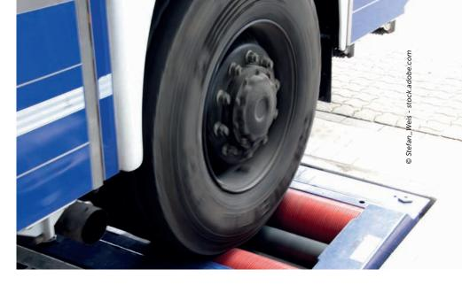
there is not the potential for a serious issue. "If we've got a bind with a pass, but can't find an obvious fault, we'll let the truck go out to work and then test it again," he explains. "Most of the time, after a laden brake test, everything is fine.
